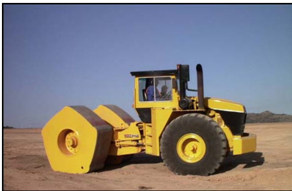
Figure 1a: A Self Propelled 5 sided 15kJ Impact Compactor
