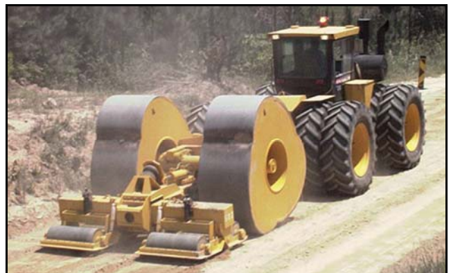
Figure 1b: A Towed 3 sided 25kJ Impact Compactor
